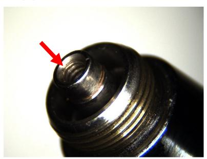
(b) Frequent disassembly may cause the sealing ring to deform or age, so it's recommended to remove the nozzle during cleaning and clean it thoroughly.
